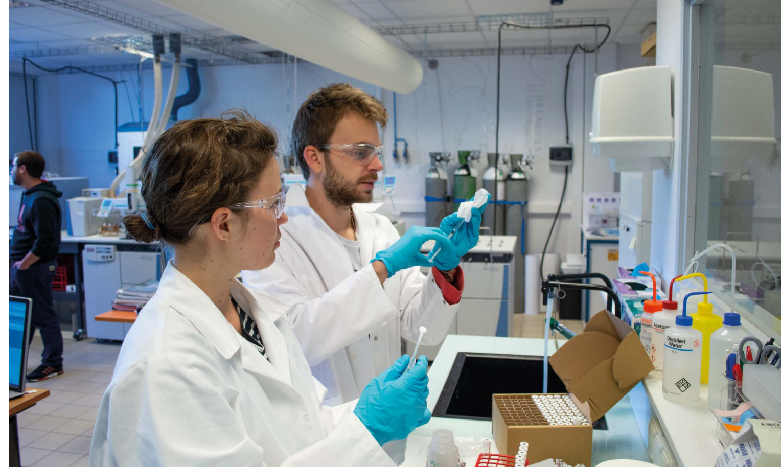
▲ The Pôle de Spectrométrie Océan (PSO), a shared facility, enables the ISblue community to carry out large-scale projects in the geosciences and biology. Here, a PSO engineer is training a master's student in the preparation of samples for mass spectrometry analysis.
